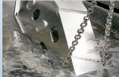
CORROSION PROTECTION – HOT DIP GALVANIZING AND PAINTING
